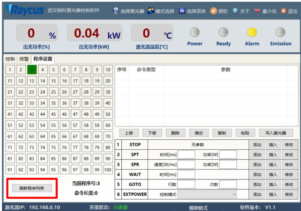
Figure 30 Checking the number of saved waveforms
