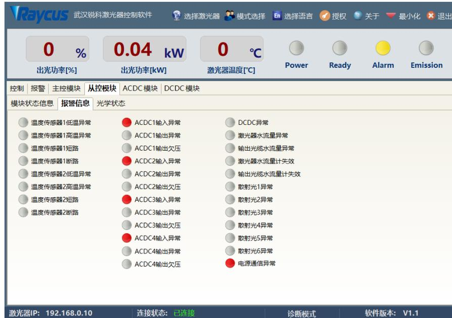
Figure 20 Slave control module alarm information interface
