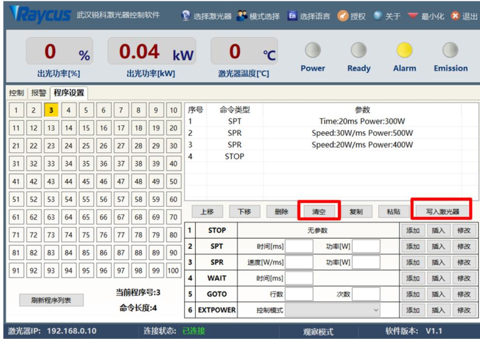
Figure 32 Clearing waveform
